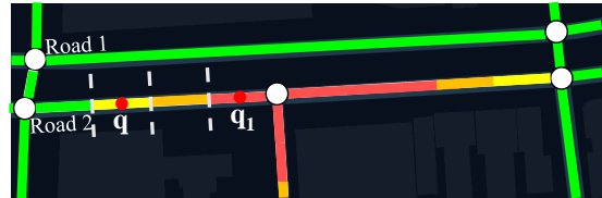
Figure 4: The 300m road (Road 2 in Figure 3) is segmented into four basic units (with 75m), called lixels. Each lixel is colored based on the kernel aggregation function, where the red color and green color denote the highest and lowest density values, respectively.
